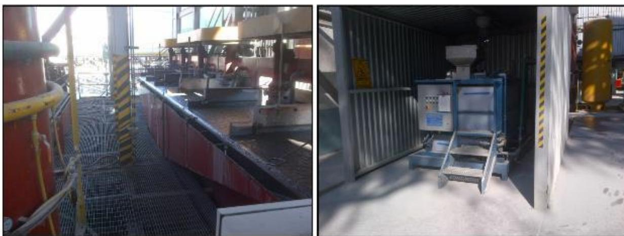
**Figure 17-6 1st Cleaner Cells (left); Flocculent Mixing System (right)**
