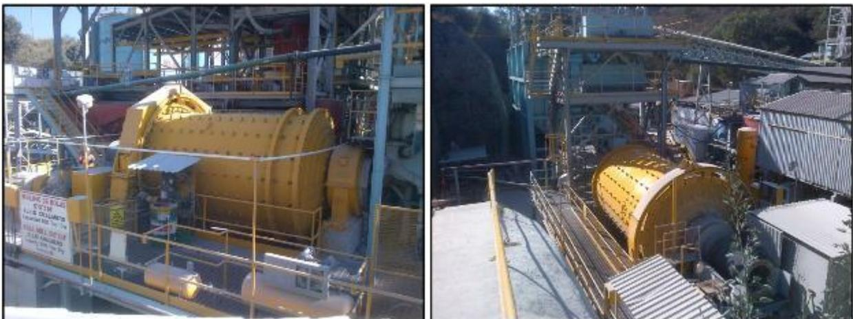
**Figure 17-5 Original Ball Mill #1, size 9'6"x14' (left), Ball Mill #2, size 11'x18'7", 1000 HP Motor, and Fine Ore Bin on the back, Both Installed in 2011 (right)**
