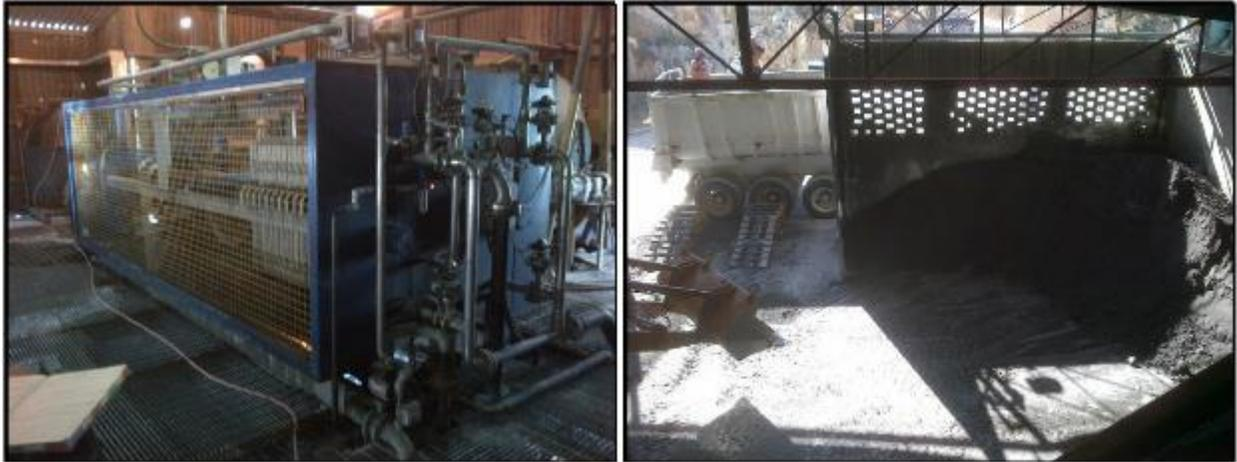
Figure 17-7 Filter Press (left); Concentrate Storage and Shipment Loading Area (right)
