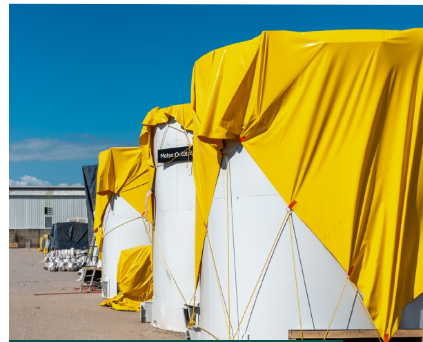
Flotation cell tanks arrived at laydown warehouse
