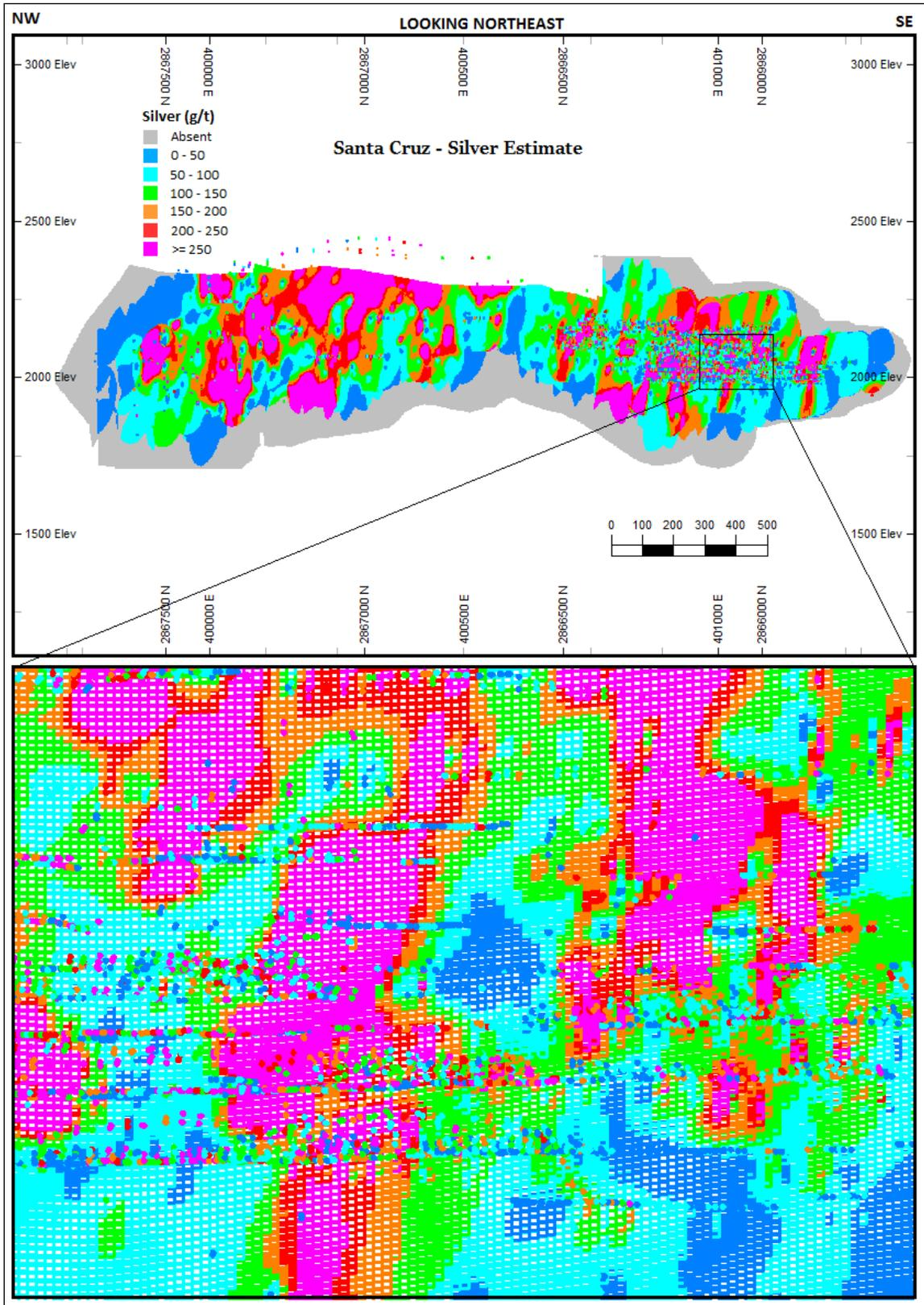
Figure 14-12 Long Section view of Santa Cruz Vein Block Model showing the Estimated Silver Grades and Composites
