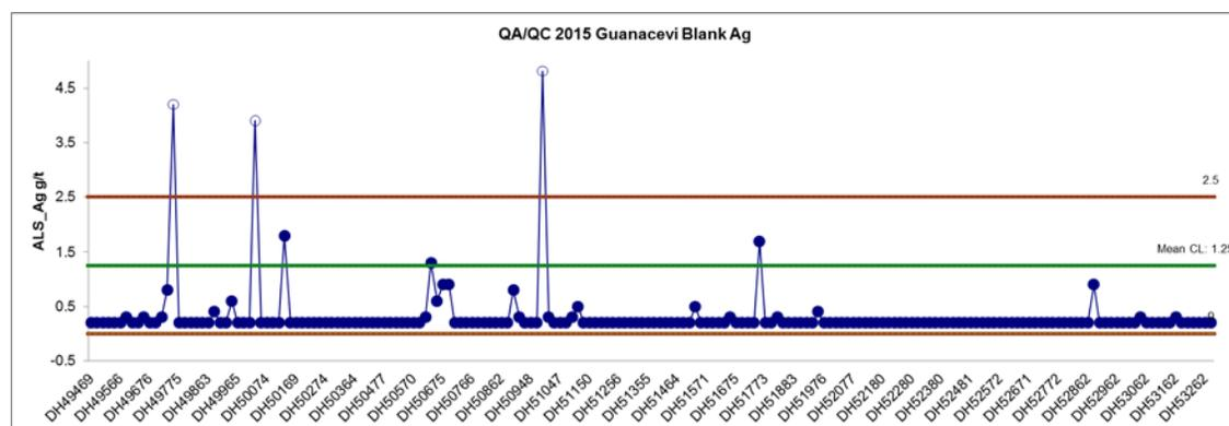
Figure 11-11 Control Chart for Silver Assay from the Blank Samples Inserted into the Sample Stream
