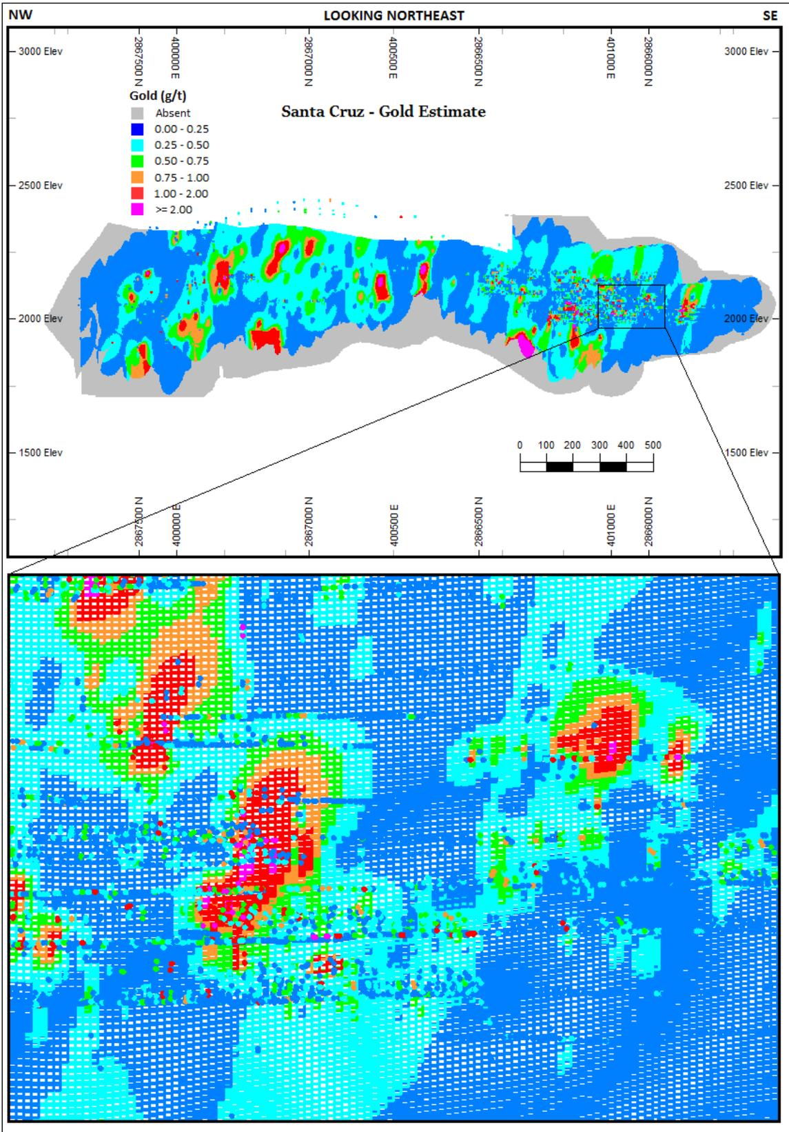
Figure 14-13 Long Section view of Santa Cruz Vein Block Model showing the Estimated Gold Grades and Composites
