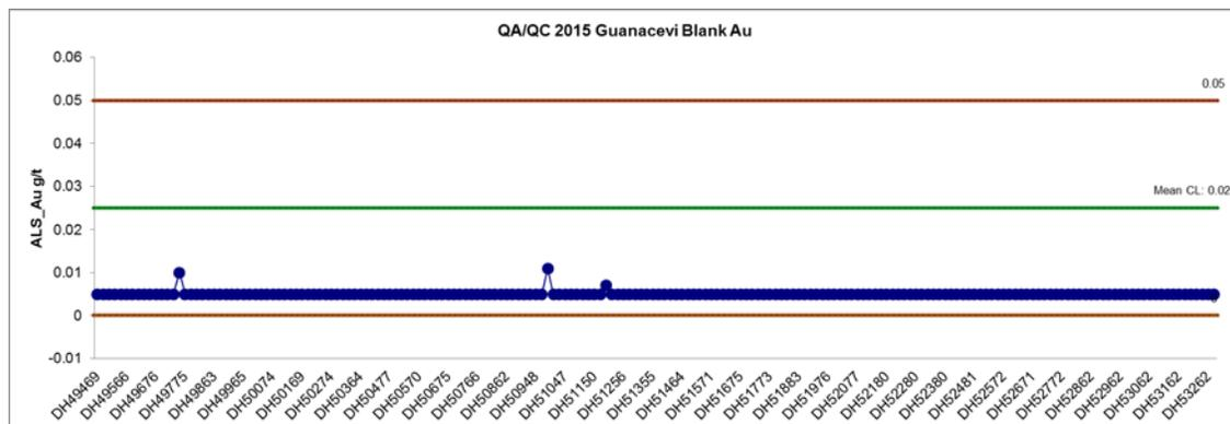
Figure 11-10 Control Chart for Gold Assay from the Blank Samples Inserted into the Sample Stream
