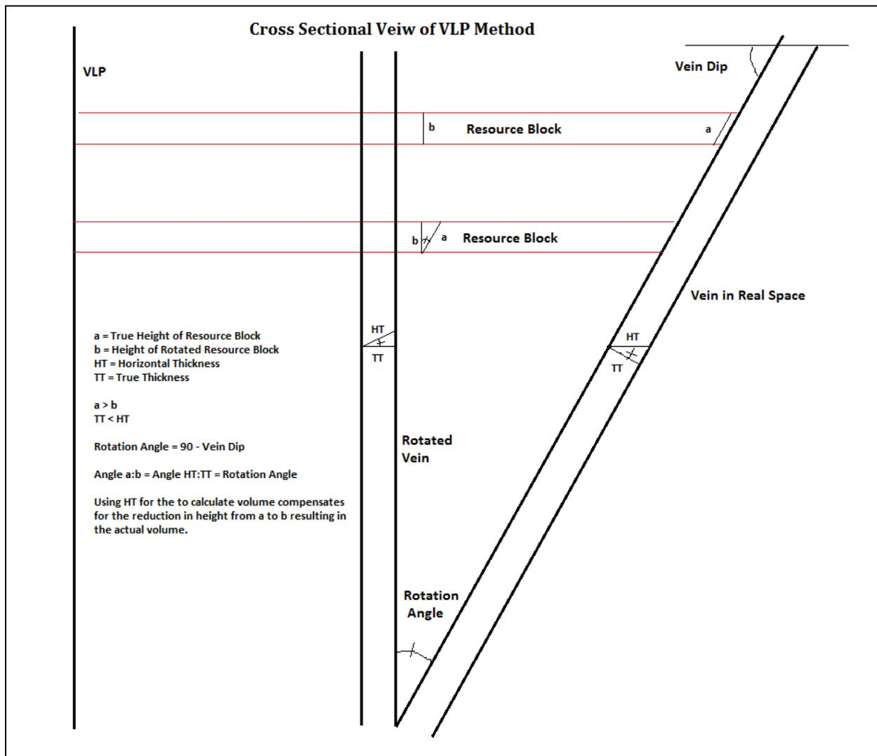
Figure 14-2 Cross Section Diagram of VLP Method
