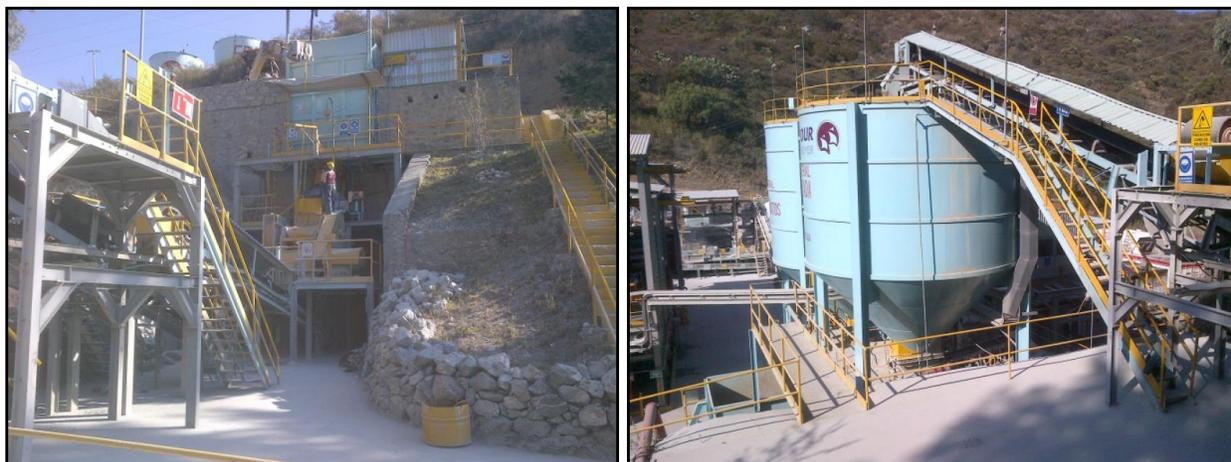
Figure 17-3 View of the Primary Crusher Circuit (left); Crushed Ore Bins (right)
