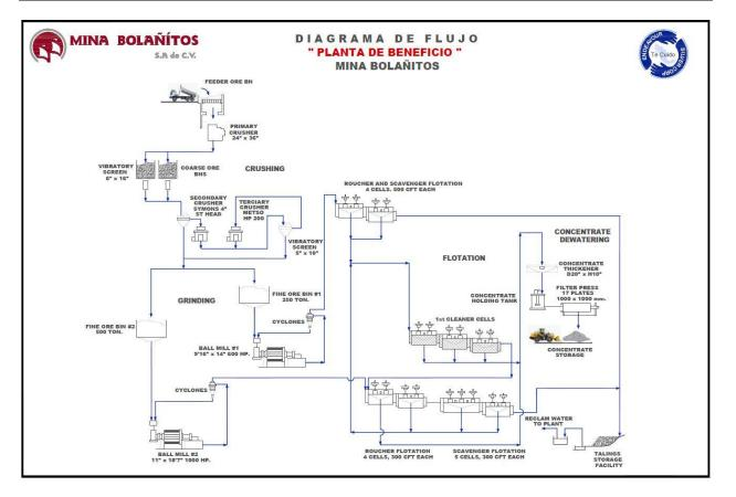
Figure 17-2 Process Flow Sheet of the Bolañitos Plant
