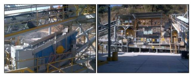
Figure 17-4 Vibration Screen, Single 6'x16'Deck (left); Fine Crushing Circuit (right)
