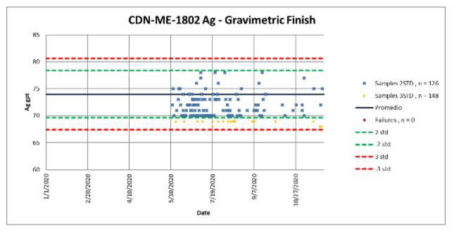
Figure 11-6 Certified Standard 1802 Silver Results – Fire Assay Gravimetric Finish
