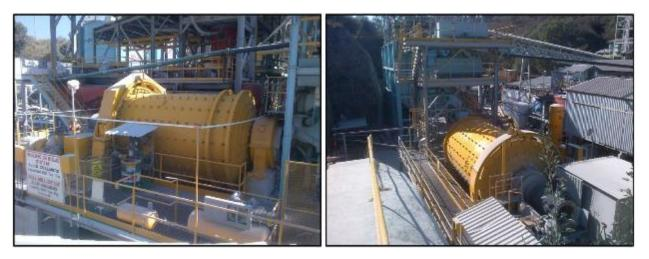
Figure 17-5 Original Ball Mill #1, size 9'6"x14' (left), Ball Mill #2, size 11'x18'7", 1000 HP Motor, and Fine Ore Bin on the back, Both Installed in 2011 (right)
