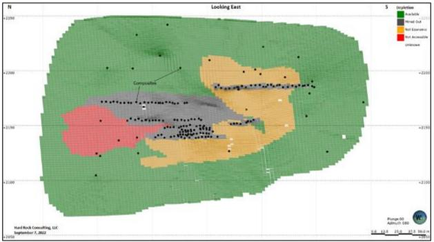
Figure 14-16 Depletion Codes for the CEC1 Vein
