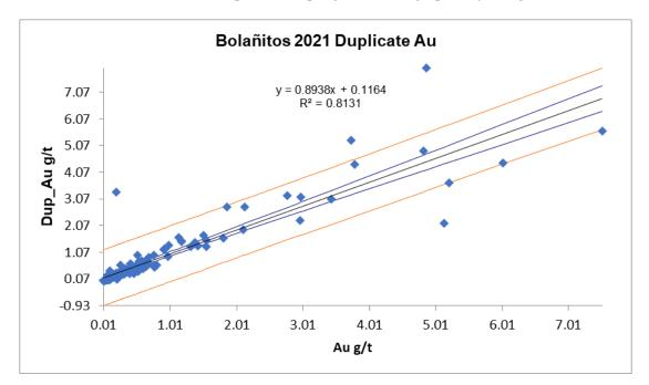
Figure 11-10 Performance of Field Duplicates for Gold from Endeavour Silver's Bolañitos Drilling Program
