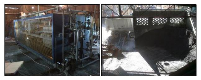
Figure 17-7 Filter Press (left); Concentrate Storage and Shipment Loading Area (right)
