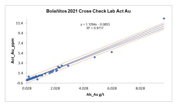
Figure 11-24 Scatter Plot of Check Assays for Gold (SGS vs ALS)
