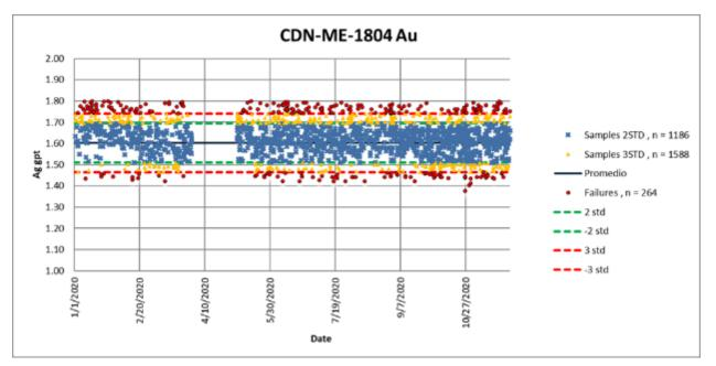
Figure 11-10 Certified Standard 1804 Gold Results – Fire Assay Gravimetric and AA Finish Combined
