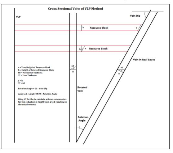
Figure 14-2 Cross Section Diagram of VLP Method
