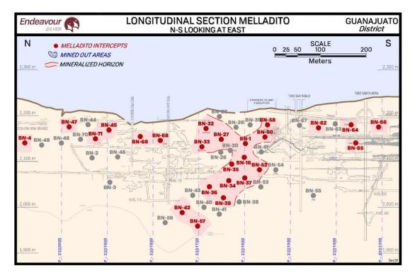
Figure 10-3 Longitudinal Section (looking E) showing intersection points on Melladito vein.
