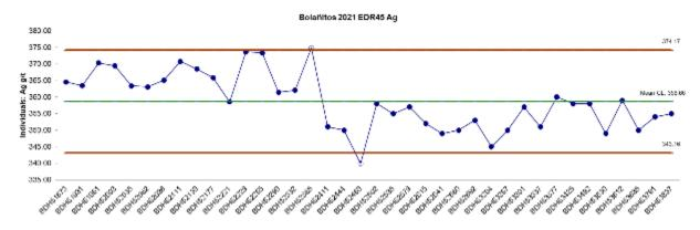
Figure 11-18 Control Chart for Silver Assays from the Standard Reference Sample EDR-45
