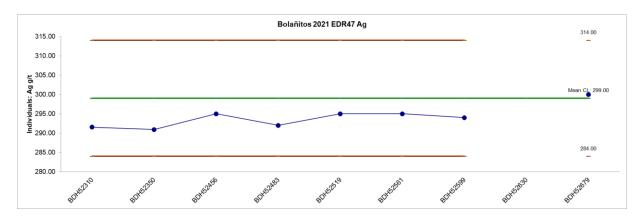
Figure 11-20 Control Chart for Silver Assays from the Standard Reference Sample EDR-47
