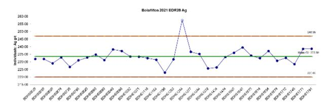
Figure 11-14 Control Chart for Silver Assays from the Standard Reference Sample EDR-39
