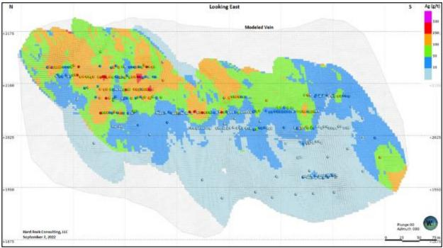
Figure 14-13 Long Section view of PLT1 Vein Block Model showing the Estimated Silver Grades and Composites
