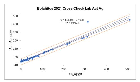
Figure 11-25 Scatter Plot of Check Assays for Silver (SGS vs ALS)
