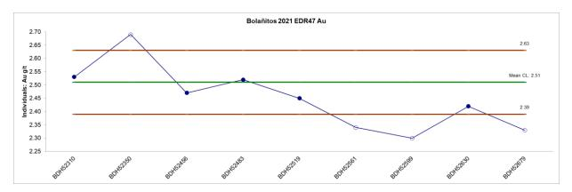
Figure 11-19 Control Chart for Gold Assays from the Standard Reference Sample EDR-47
