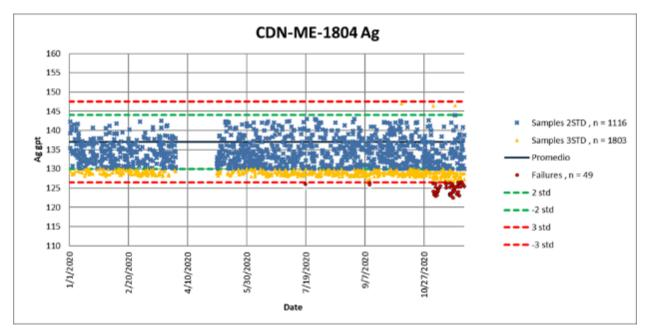
Figure 11-9 Certified Standard 1804 Silver Results – Fire Assay Gravimetric and AA Finish Combined
