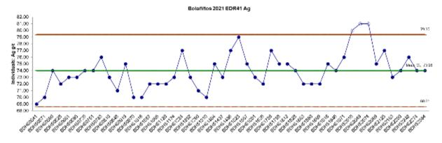
Figure 11-16 Control Chart for Silver Assays from the Standard Reference Sample EDR-41
