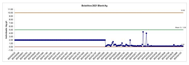
Figure 11-9 Control Chart for Silver Assay from the Blank Samples Inserted into the Sample Stream
