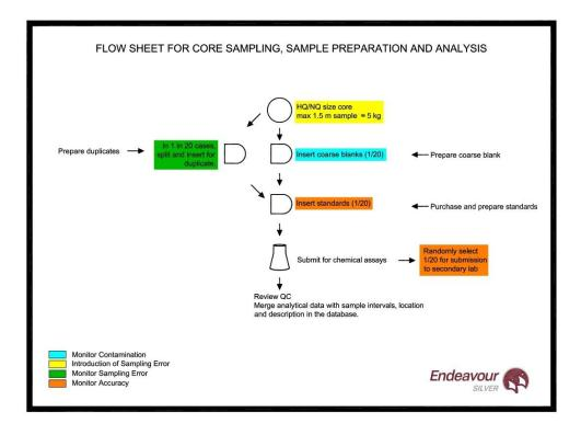
Figure 11-7 Flow Sheet for Core Sampling, Sample Preparation and Analysis
