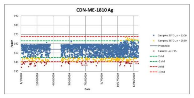
Figure 11-11 Certified Standard 1810 Silver Results – Fire Assay Gravimetric and AA Finish Combined
