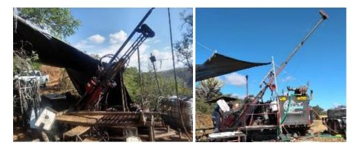
Figures 10-15 & 10-16 In-house drill rig in pad for drill hole BS-05 (Tepetateras-Lulú) and Versa drill rig in pad for drill hole BS-19 (Tepetateras-Lulu).
