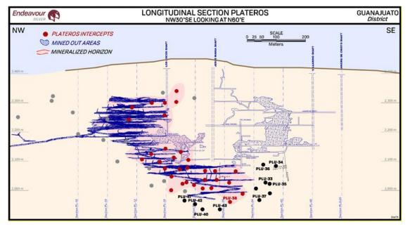
Figure 10-7 Longitudinal Section (looking NE) showing intersection points on Plateros vein.
