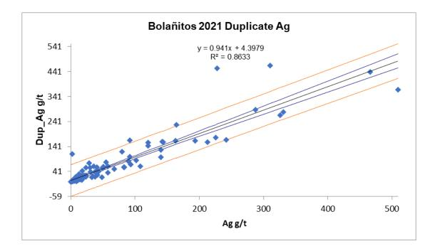
Figure 11-11 Scatter Diagram of the Silver Re-Assayed ALS Samples
