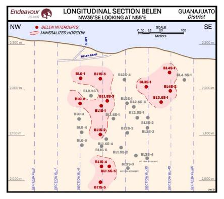
Figure 10-11 Longitudinal Section (looking NE) showing intersection points on Belen vein.
