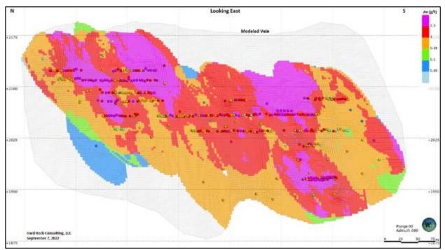
Figure 14-14 Long Section view of PLT1 Vein Block Model showing the Estimated Gold Grades and Composites
