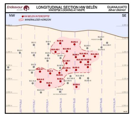
Figure 10-10 Longitudinal Section (looking NE) showing intersection points on Hw Belen vein.
