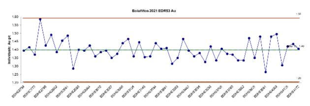
Figure 11-21 Control Chart for Gold Assays from the Standard Reference Sample EDR-53
