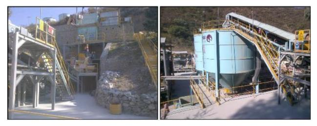
Figure 17-3 View of the Primary Crusher Circuit (left); Crushed Ore Bins (right)
