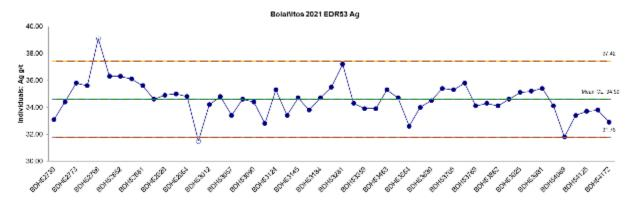
Figure 11-22 Control Chart for Silver Assays from the Standard Reference Sample EDR-53
