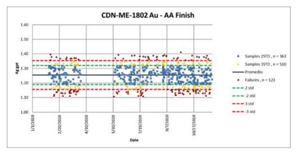
Figure 11-7 Certified Standard 1802 Gold Results – Fire Assay AA Finish
