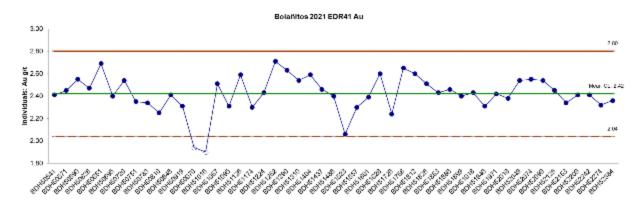
Figure 11-15 Control Chart for Gold Assays from the Standard Reference Sample EDR-41
