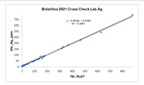
Figure 11-23 Scatter Plot of Check Assays for Silver (ALS vs SGS)
