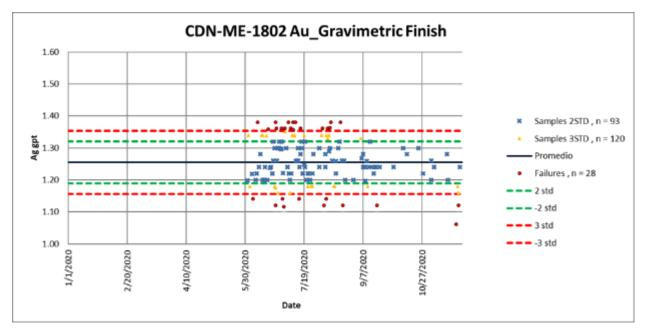
Figure 11-8 Certified Standard 1802 Gold Results – Fire Assay Gravimetric Finish
