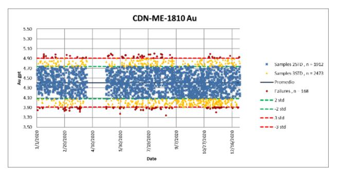
Figure 11-12 Certified Standard 1810 Gold Results – Fire Assay Gravimetric and AA Finish Combined
