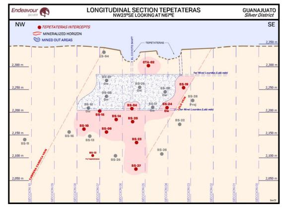
Figure 10-20 Longitudinal Section (looking NE) showing intersection points on Tepetateras vein.
