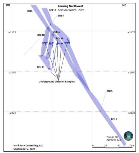
Figure 14-3 Cross Section of Bolañitos Veins Set showing Drillhole and Channel Sample Selections.
