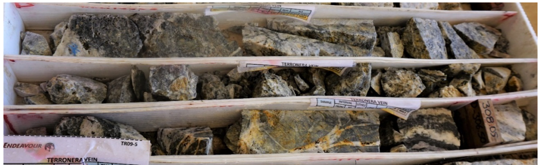
Figure 12-1: Drill Hole TR09-5, 306 to 308.10 m, illustrating breccia with bands of strong silicification, strong sulphide mineralized zone, crystals of argentite, galena, chalcopyrite, and pyrite disseminated. Weak oxidation. (prepared by Wood, dated 2021)
