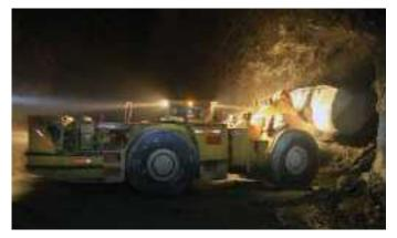
A scoop tram loading ore at Bolañitos
